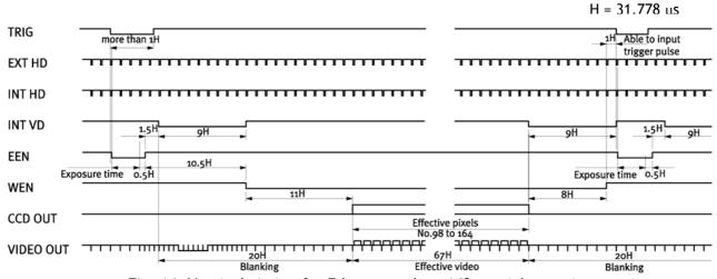
Fig. 14. Vertical timing for Edge pre-select 1/3 partial scanning
